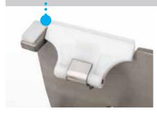
The scraping effect on the cylinder surface resulting in a extremely high heat rate efficiency as well as a high energy saving is given by the strength of the materials the scrapers are made of, their special inclination on the touch point and the specific high-thrust spring. Scrapers' material is provided with EC marking for use in food handling equipment.
