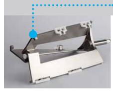
Special design helicoidal stirrer with blade variable convergence and high-performance scrapers: these are only few of the features marking out the new stirrer. A perfect batch freezing is the result of a systematic and uniform spreading of gelato on the whole cylinder surface thus avoiding the excessive freezing of gelato on the blades or in the middle of the cylinder.
